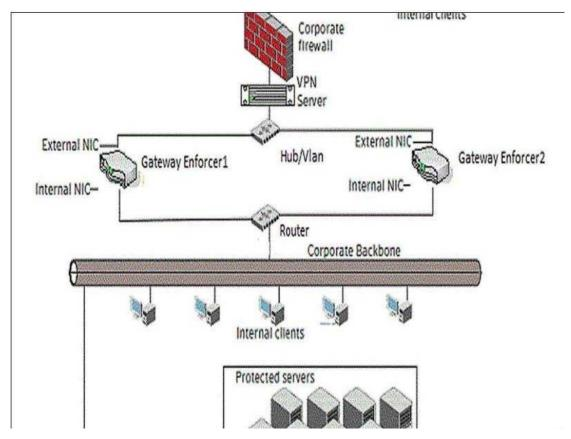
A Symantec Network Access Control administrator is trying to implement two Gateway Enforcers in failover mode. The administrator has implemented the two Enforcers in the network as shown in the exhibit. After starting both Gateway Enforcers, the administrator finds that both Enforcers are in active mode. What is the likely cause of the problem?
