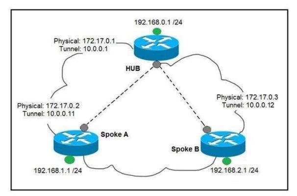
A interface Tunnel0 description mGRE – DMVPN Tunnel ip address 10.0.0.11 255.255.255.0 ip nhrp map multicast dynamic ip nhrp network-id 1 tunnel source 10.0.0.1 tunnel destination FastEthernet 0/0 tunnel mode gre multipoint Download Full Version 300-410 Exam Dumps (Updated in Feb/2023)
