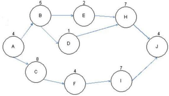
Based on the project network diagram, how much float is available for Activity H if Activity B is delayed by four days and Activity D is delayed by two days?
