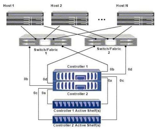
In the diagram shown, a portset is created on controller 1 with the command:
