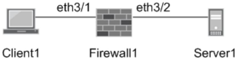
In the exhibit, eth3/1 is in the client-vr virtual router and eth3/2 is in the server-vr virtual router. Your policies permit all traffic between all zones. You want to ensure Client1 can contact Server1.
