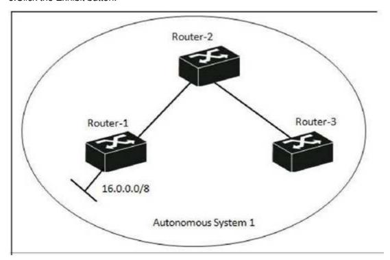
Router-1 and Router-2 are BGP peers. Router-2 and Router-3 are BGP peers. However, Router-3 has not
