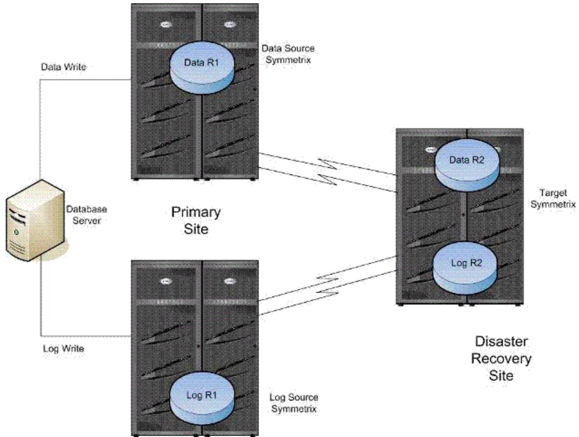
A. An SRDF failover would be initiated on all volumes and processing would automatically be switched over to the disaster recovery site.
