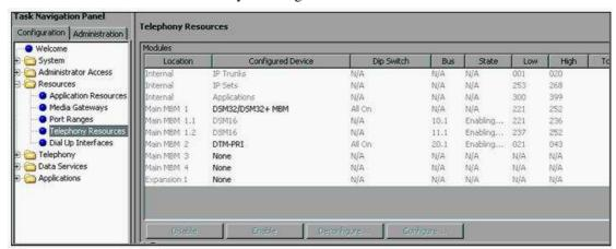
A.Select the row of the DTM you configured. Click the Configure button and enter DTM-T1 as the module type.
