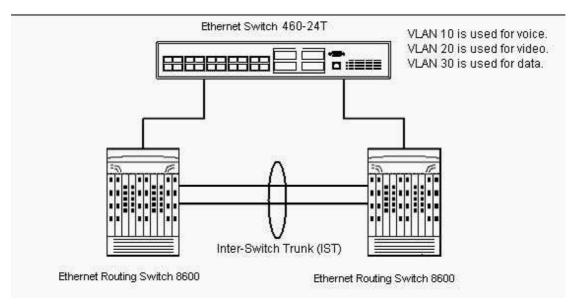
A.Configure MLT on the Ethernet Switch 460 and SMLT on the Ethernet Routing Switch 8600s, and tag all VLANs over these links.
