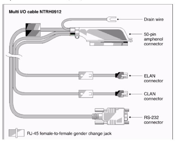
A.Connect the ELAN connector on the multi I/O cable (NTRH0912) to the ELAN hub.
