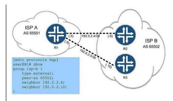
In the exhibit, ISP A is charged a higher rate for traffic sent to R2. You are asked to lower costs for ISP A by configuring R1 to send traffic to R3 whenever possible.
