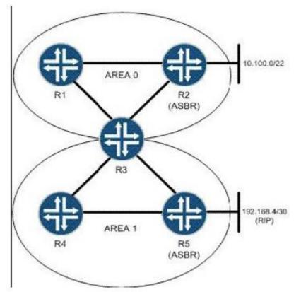
You are asked to configure an OSPF network based on the topology shown in the exhibit. You must keep the link-state database in Area 1 as small as possible. What will accomplish this? A. Area 0 should be configured as a stub area so that it will not announce routes into Area 1.
